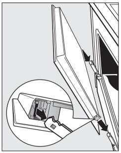
■ Hold the door securely at both sides and carefully fit it back onto the hinge guides.
